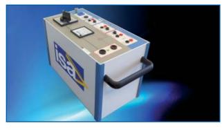
The option allows performing both the measurement of: soil resistivity, ground grid resistance, step and touch tests, and of: overhead lines zero sequence and mutual coupling coefficients. This option applies to STS 5000 and 4000 models.
