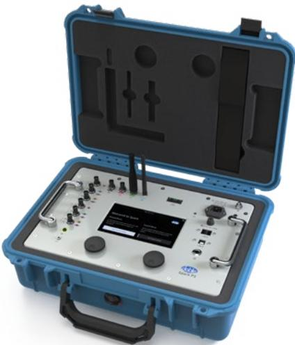
The Doble Spark P3 is the most universal PD and EMI analyzer available today. It utilizes a combination of various signal processing technologies that enable the user to identify the characteristics of insulation system deterioration that could lead to the failure of high voltage equipment in the field and in the laboratory. The Spark P3 enables the user to utilize any sensor capable of detecting PD, with its detectors covering frequencies from 9kHz to 2GHz.
